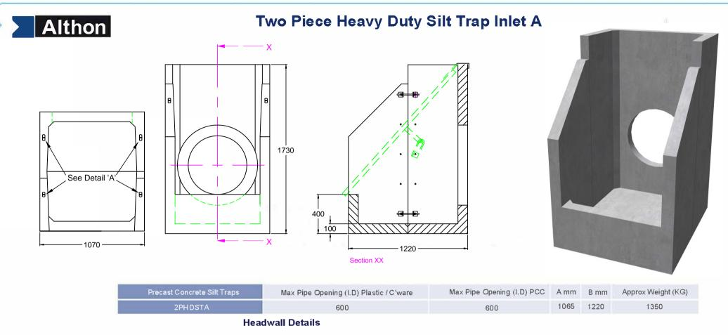
Althon 2 Piece Heavy duty silt Traps are sturdy structures for use on large diameter pipes and are ideally suited for use in water courses with high velocities of water flow. Althon provide as standard with each unit a galvanized weed screen and removable centre panel for access to the silt for cleaning. Lifting points are cast into the wingwalls for safe handling with Althon Lifting Clutches.
