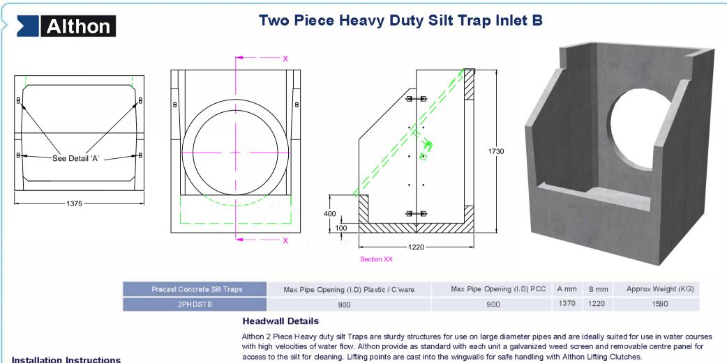
1. Dig out the bank of the watercourse to take the appropriate size of the headwall making sure that the headwall will not protrude into the path of the water flow.
