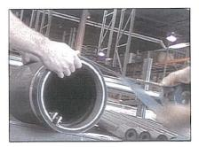
Step 6: Unroll more of the tape. Remove plastic from tape. Continue to apply tape to the outside circumference of the valve to build up the O.D. to the desired size. In this example, 3-4 layers of continuously wrapped tape was used. The number of layers required is a function of the pipe I.D. dimension.
