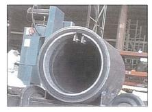
Step 12: Once the bolts are tightened and the rubber tape is compressed, the CheckMate<sup>TM</sup> Valve is installed and ready for operation.
