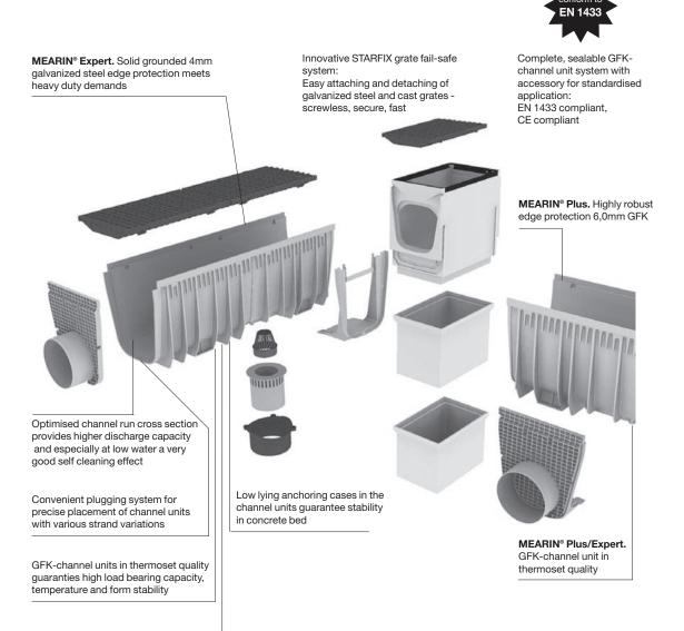
High stability of channel units opens a huge field of deployment up to drainage
