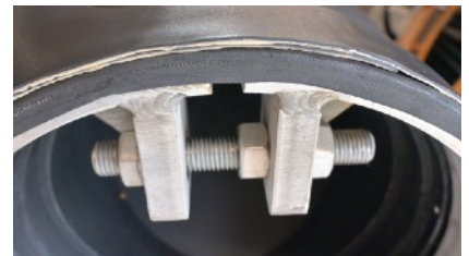
Check the valve O.D. snugly fits within the pipe I.D.
