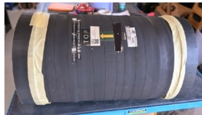
Apply tape around the valve cuff clamp end
