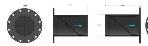
Flanged models connect to mating flanges on existing pipes. There is no difference in the pressure rating of the flanged models compared to the IDP models.
