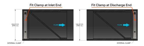
The expanding C-Clamp of the Check-Flex® G5 valve can used in either the Inlet End or the Discharge End of the valve.
