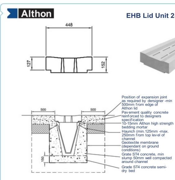
The EHB lid unit has been designed for use in areas trafficked by articulated HGV vehicles.
