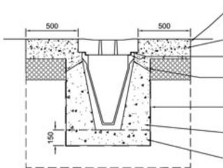
Position of expansion joint as required by dersigner -min 500mm from edge of Althon lid Pavement quality concrete reinforced to designers specification 10-15mm Althon high strength bedding mortar
