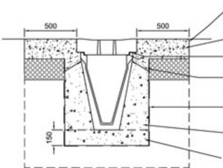
Position of expansion joint as required by dersigner -min 500mm from edge of Althon lid
