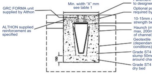
Pavement quality concrete to designers specification Optional position of joint as required by designer
