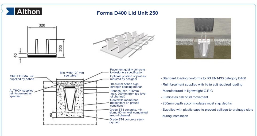
The FORMA lid has been designed for use in hevay duty industrial areas, e.g. distribution depots, dock areas, service yards etc. The Forma lid has been tested to D400 loading as standard.
