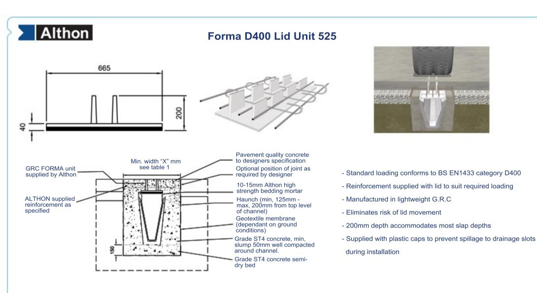
The FORMA lid has been designed for use in hevay duty industrial areas, e.g. distribution depots, dock areas, service yards etc. The Forma lid has been tested to D400 loading as standard.
