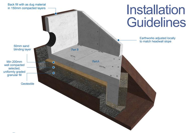
Ensure that first or last spigot/butt or socket/butt pipe that is to be fitted to the Headwall is in position and free from backfill.
