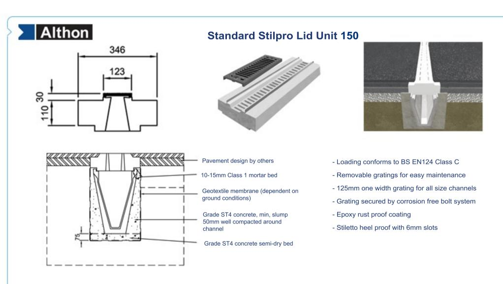
The STILPRO Lid was developed in conjunction with landscape architects who expressed a requirement for a standard width cast iron stiletto heel proof grating, whilst utilising the benefits of incorporating an ALTHON High Capacity Channel. The remainder of the lid unit is covered by asphalt or macadam.
