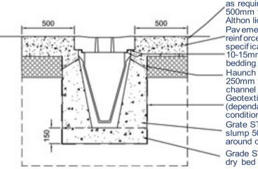
Position of expansion joint as required by dersigner -min 500mm from edge of Althon lid Pavement quality concrete reinforced to designers specification 10-15mm Althon high strength bedding mortar Haunch (min.125mm -max. 250mm from top level of channel Geotextile membrane (dependant on ground conditions)
