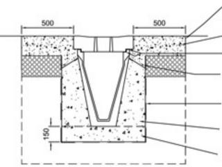
Position of expansion joint as required by dersigner -min 500mm from edge of Althon lid Pavement quality concrete reinforced to designers specification 10-15mm Althon high strength bedding mortar Haunch (min.125mm -max. 250mm from top level of channel Geotextile membrane (dependant on ground conditions)
