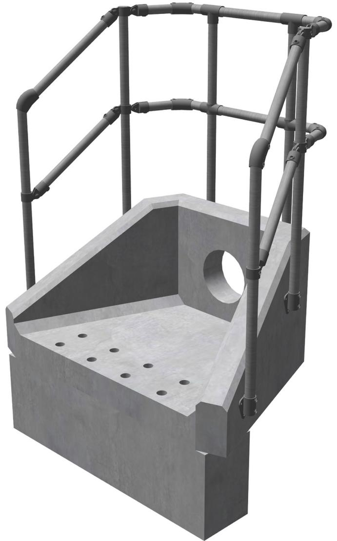
We are able to cast onto the apron of the basin inlet headwalls stepped baffle blocks for when the velocity of the discharge needs to be dissipated before it enters the watercourse.
